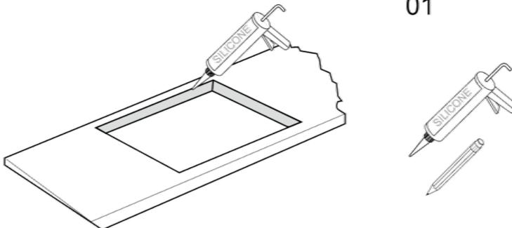
Cut out worktop to supplied dimensions shown (fig. 1) with suitable equipment. Seal the cut edge of the worktop using silicone or PTFE and allow to dry prior to fitting the hob.
