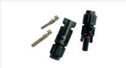
MC4 DC Solar Cable Connectors For cables 2.5mm 2 to 6.0mm 2 , 30A max current, max voltage 1000V. IP68.
